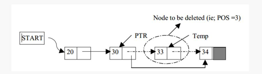
Suppose START is the first position in linked list. Let DATA be the element to be deleted. TEMP and PTR are temporary pointers to hold the node address.
